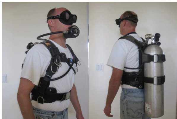
Good Hose Arrangement with 48” 2 nd Stage
