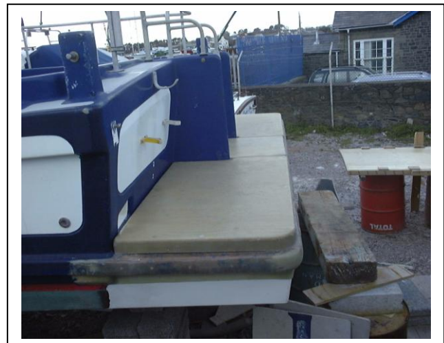
The finished hatches (minus Gel coat), in position on the swim platform. These hatches will be bolted down and will sit on rubber seals. The starboard side has the boarding/dive ladder through bolted.
