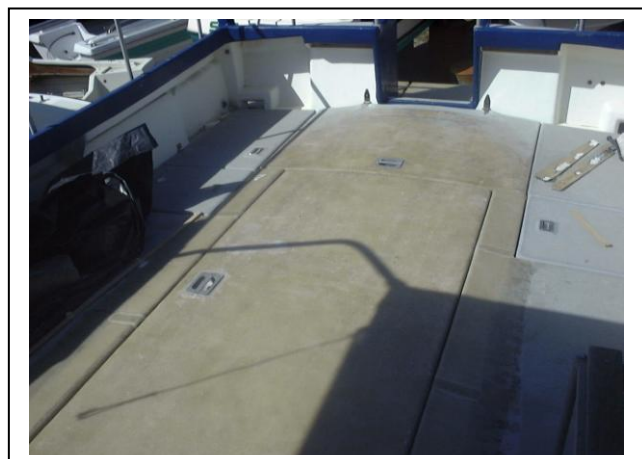
The two hatches in place on the deck. Note the new "home made" heavy-duty flush handles.
