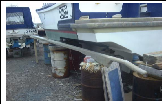
The complete keel shoe (upside down) sits alongside of the boat. The bow end has been added since completion of the forward false keel (see page 9).
