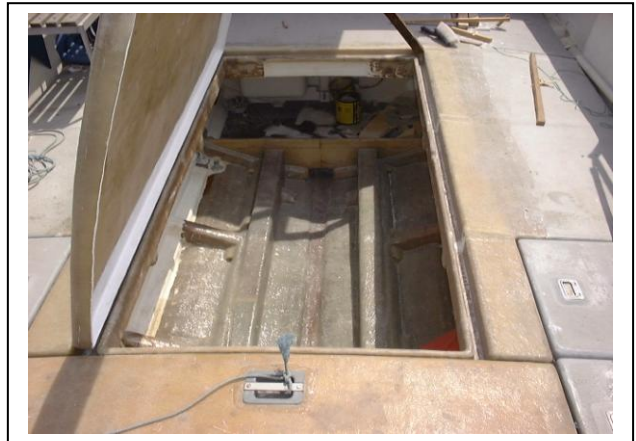
After gelling and sanding the outside of the keel shoe it has been stuck on with mucho wet gel. Lots of little bent sticks apply steady pressure after an initial shove with two hydraulic jacks.
