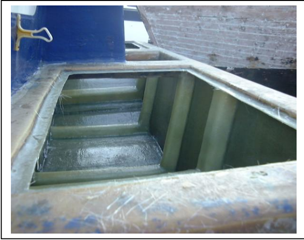
The view inside the new hull extension, seen through the swim platform, shows that the stringers continue up the new transom.
