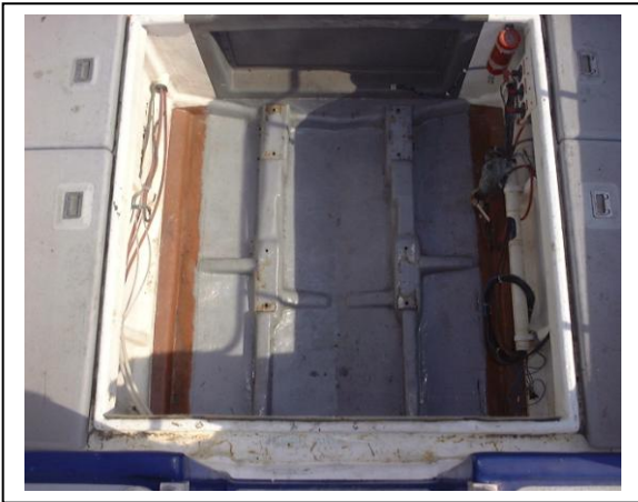
Inside the old stern engine compartment, now sadly empty. Note the soon to prove problematic engine beds.
