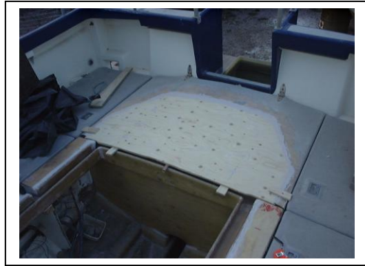
The old engine hatch (now the fish/gear hold hatch) with the new half-inch shuttering ply piece spliced in place.
