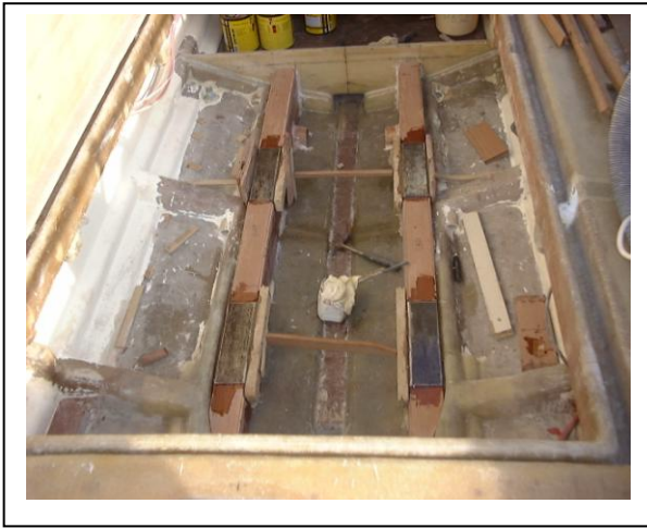
The ply tops of the beds are bedded down on gel with the 20mm steel plates bedded on wet mat.
