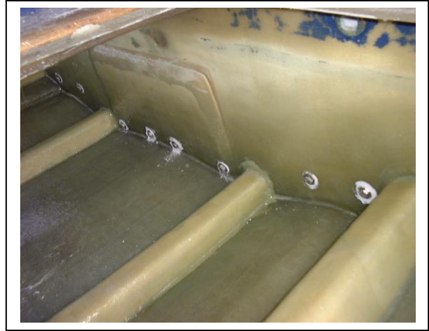
Belt and Braces - 8 stainless bolts pass, low down, through the new hull moulding and the old transom.
