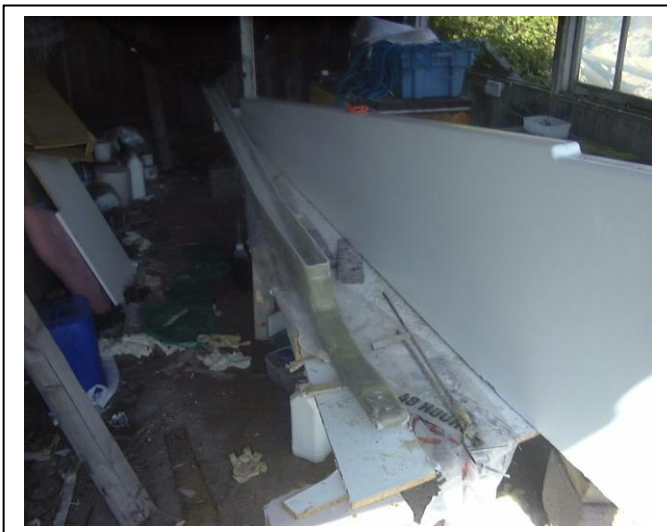
The complete shoe and skag, now trimmed up, lie next to the upside down keel, which is devoid of its protective polythene.
