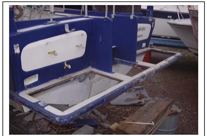
Meanwhile, back at the boat. Panels were cut from the swim platform to facilitate access. The 2 outer ones were saved to be glassed back in place later. A lip was glassed around the edge from underneath (upside down glassing – my favourite job!). Central hole will be a hatch.
