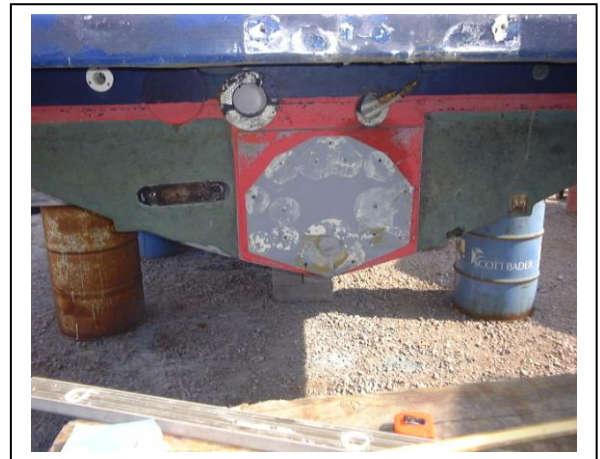
Remove all stern gear, exhaust, anodes etc and mark out the cutting lines with a permanent felt pen.
