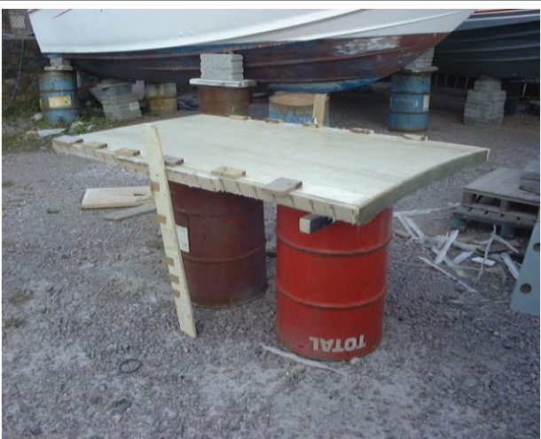
The new engine hatch is made from 90% of an 8 x 4 sheet of half-inch shuttering ply. Shown is the sheet with formica edge shuttering in place. Getting the curve to match the camber of the deck is tricky. Six coats of glass will finish the job.
