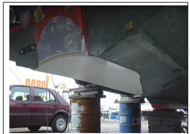
Removing the former reveals the new prop tunnel under the stern hull. Looks good.
