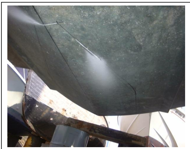
Inside the old stern engine compartment, now sadly empty. Note the soon to prove problematic engine beds.
