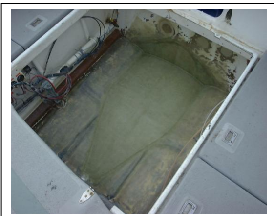
Three complexes on top of two coats of Gel. Hey, now my boat would float again. If only I had an engine.
