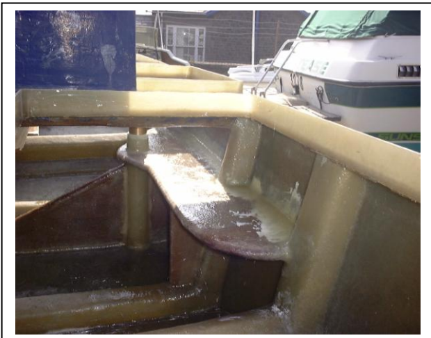
The ply tops of the beds are bedded down on gel with the 20mm steel plates bedded on wet mat.
