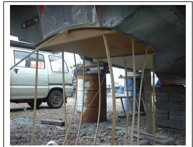
The former is held in place by "springy" sticks of wood. This stops the hardboard coming loose when working on the boat.
