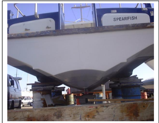
The view beneath the new transom reveals the new, substantial, prop tunnel.
