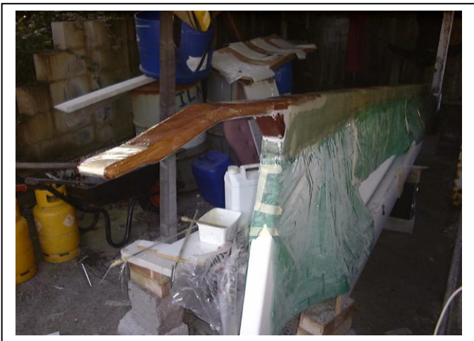
The keel/rudder skag is made of a stainless steel strip and iroko cladding. Two bolts are made captive by welding.
