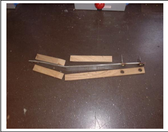
The keel/rudder skag is made of a stainless steel strip and iroko cladding. Two bolts are made captive by welding.
