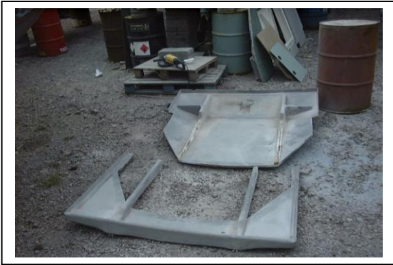
The old engine hatch (upside down) was cut in two. The piece nearest to camera is to be reused.
