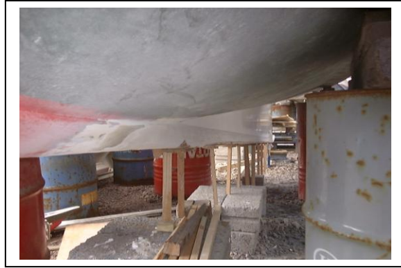
After gelling and sanding the outside of the keel shoe it has been stuck on with mucho wet gel. Lots of little bent sticks apply steady pressure after an initial shove with two hydraulic jacks.
