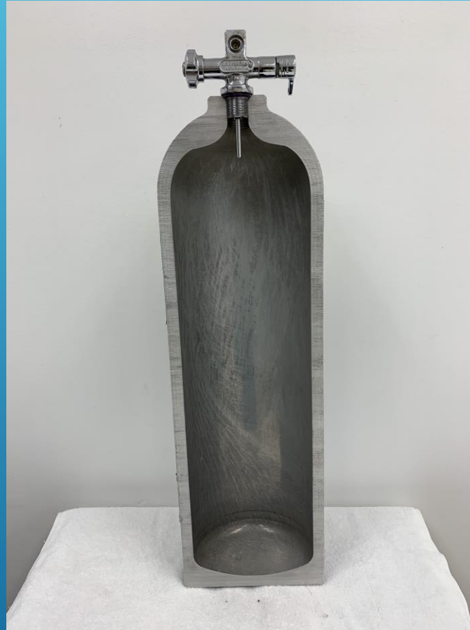
Aluminum Tank cut-in-half with Vintage Valve
